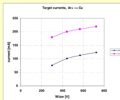
FIG.3: Target currents of the Dual Target Magnetron in dependence from the primary ion energy (argon,  $10^{-2}$  mbar, 80 W)
