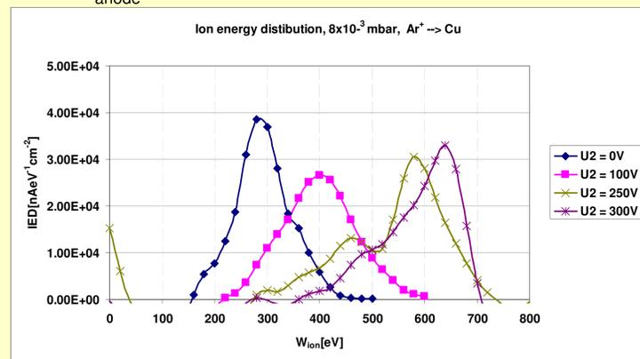
FIG. 4: Ion energy distributions of the primary ions at sputtering of copper with argon measured with a Retarding Field Analyzer arranged at target 2.
