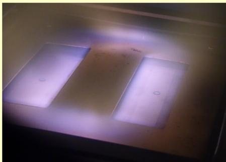
FIG.2: Dual Target Magnetron in operation (argon,  $10^{-2}$  mbar, 80 W)
