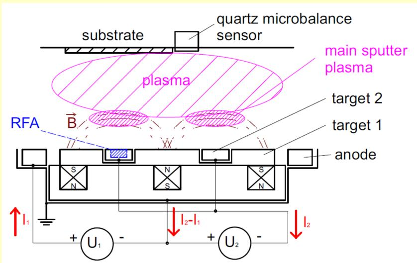
FIG.1: Principal arrangement of sputtering with the Dual Target Magnetron in cross section
