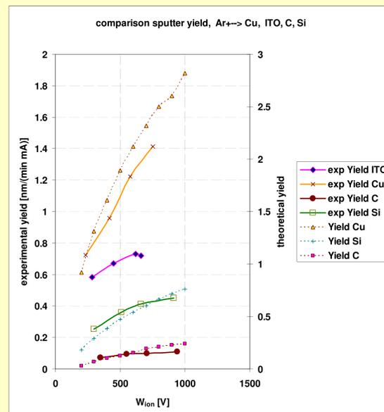
FIG. 5: Comparison of theoretical and estimated sputter yield at target 2 for different target materials in dependence on the primary ion energy.
