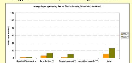
FIG.5: Energy flux analysis for sputtering with 300 eV (yellow) and 900 eV (green) primary ion energy
