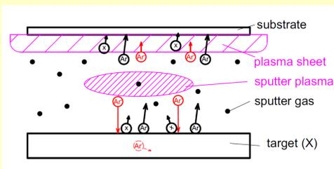
FIG.1: Schematic illustration of the energetic particles occurring in magnetron sputtering
