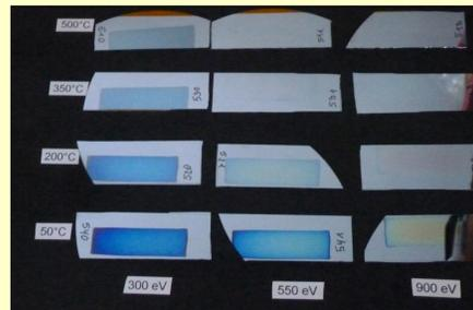
FIG.3: Overview silicon layers on crystalline silicon in dependence from temperature and primary ion energy
