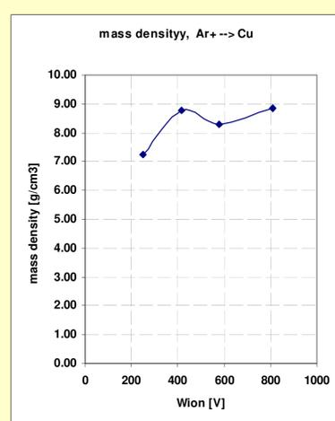
FIG.2: Specific resistance (left) and mass density (right) of copper layers in dependence from the primary ion energy sputtered with the DTM
