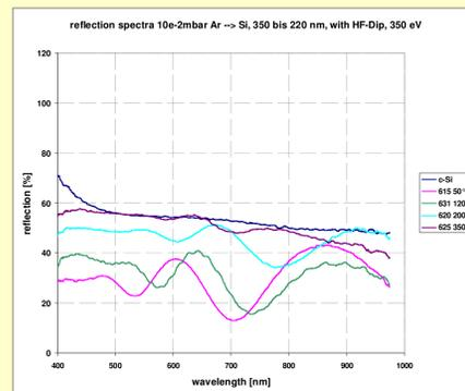
A high phosphorous doped silicon target had been used. Crystalline silicon substrates prepared with an HF-dip before deposition had been used. The substrate temperature was varied from 50°C to 500°C.
