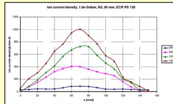
*Ion current density profiles in dependence on power*
