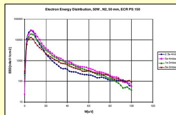
*Electron Energy Distribution in dependence on pressure on logarithmic scale*
