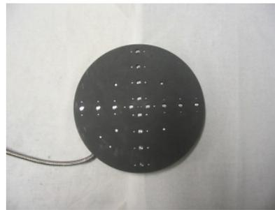
**Fig. 2.5:** Arrangement of two linear faraday cup lines for ion beam profile analysis (2 x 8 x 20 mm)
