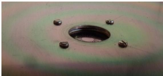
Fig.5.5.2.: Retarding Field Analyzer embedded into a substrate holder at sputtering of ITO with argon
