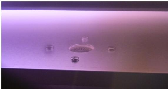
**Fig.5.2.5.:** Retarding Field Analyzer integrated into the ground electrode (0.1 mbar N<sub>2</sub>, 100 W electrode distance 40 mm)
