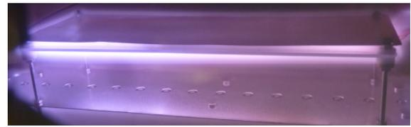
Fig.5.2.2.: Integrated plasma sheet probe (16 x 20 = 320 mm, probe see Fig.5.1.3) at the ground electrode of a 50 kHz electrode plasma
